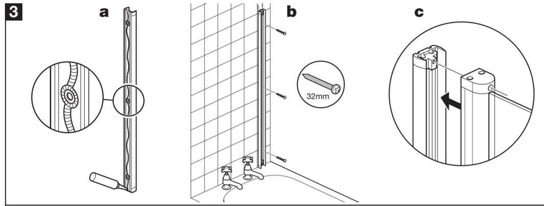
(a) Apply silicone sealant to back of wall channel as shown.
