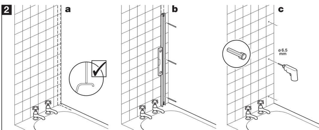
(a) Position the curtain screen on the edge of the bath ensuring the vertical profiles are supported on the bath rim.
