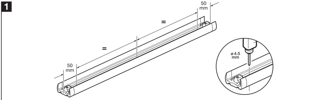
Drill three holes in the wall channel (PN80277) at points shown using a 4.5mm drill bit, through the grooved centre line.
