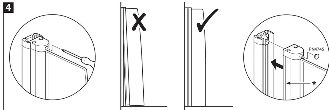
Adjust the curtain screen by tightening or loosening the top screw so that the bottom of the glass runs evenly along the bath rim. The curtain screen **MUST NOT** come out of the wall channel beyond the marked line (\*). Push fit the screw cap.
