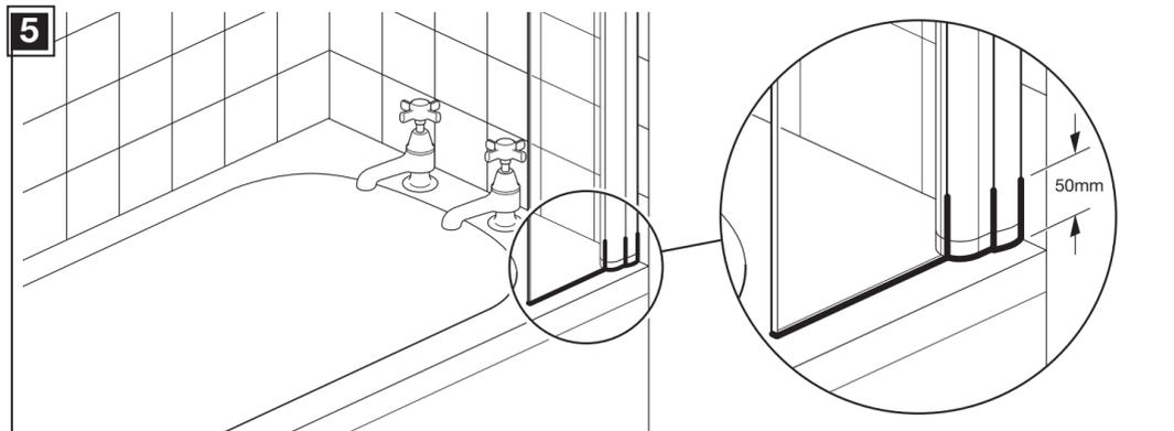
Apply silicone sealant to the outside of the curtain screen where shown. **DO NOT** apply silicone sealant to the inside face of the curtain screen.
